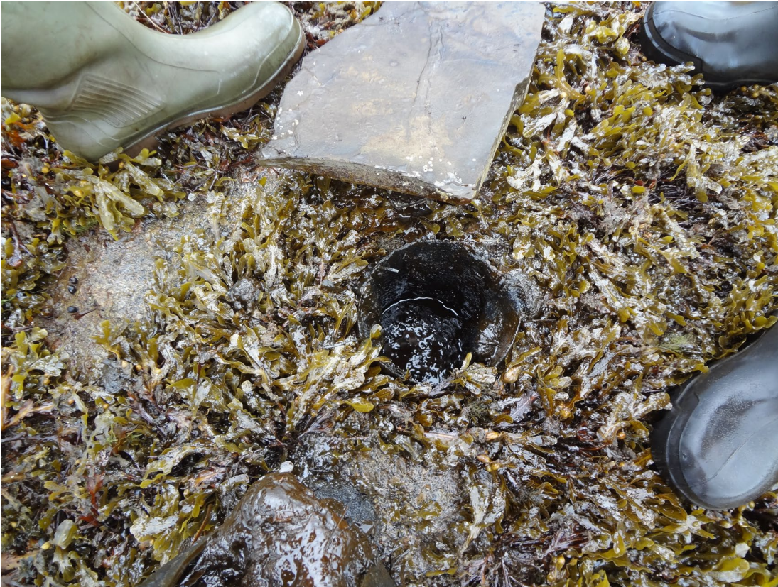
Photo 1 – Oil/Water Mixture in Casing Above Well Plug Mechanism
