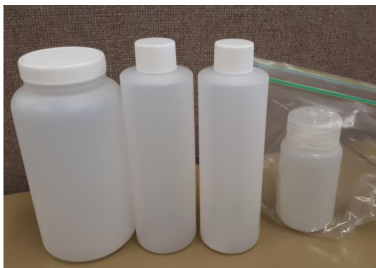
Figure 7: Bottle set for WQMA Ambient Surface Water samples
