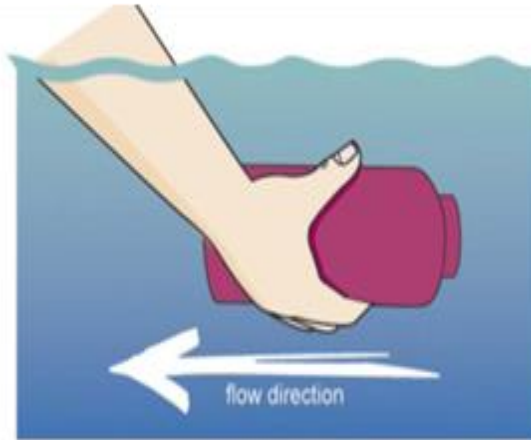
Figure 13: Example of Surface Water Sampling Technique
