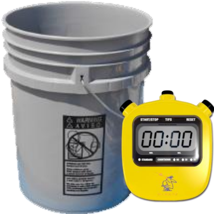
Figure 4. A bucket and stopwatch can be used to time the length of time to fill a container of known volume.
