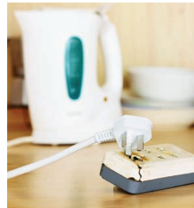
Figure 16-6 | Damaged tools and equipment may pose hazards to workers through inadequate grounding or insulation.
