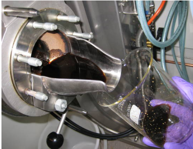
FIGURE 14. BIOREFINING OUTPUT PRODUCED FROM WOOD BY A MOBILE FAST PYROLYSIS UNIT.
