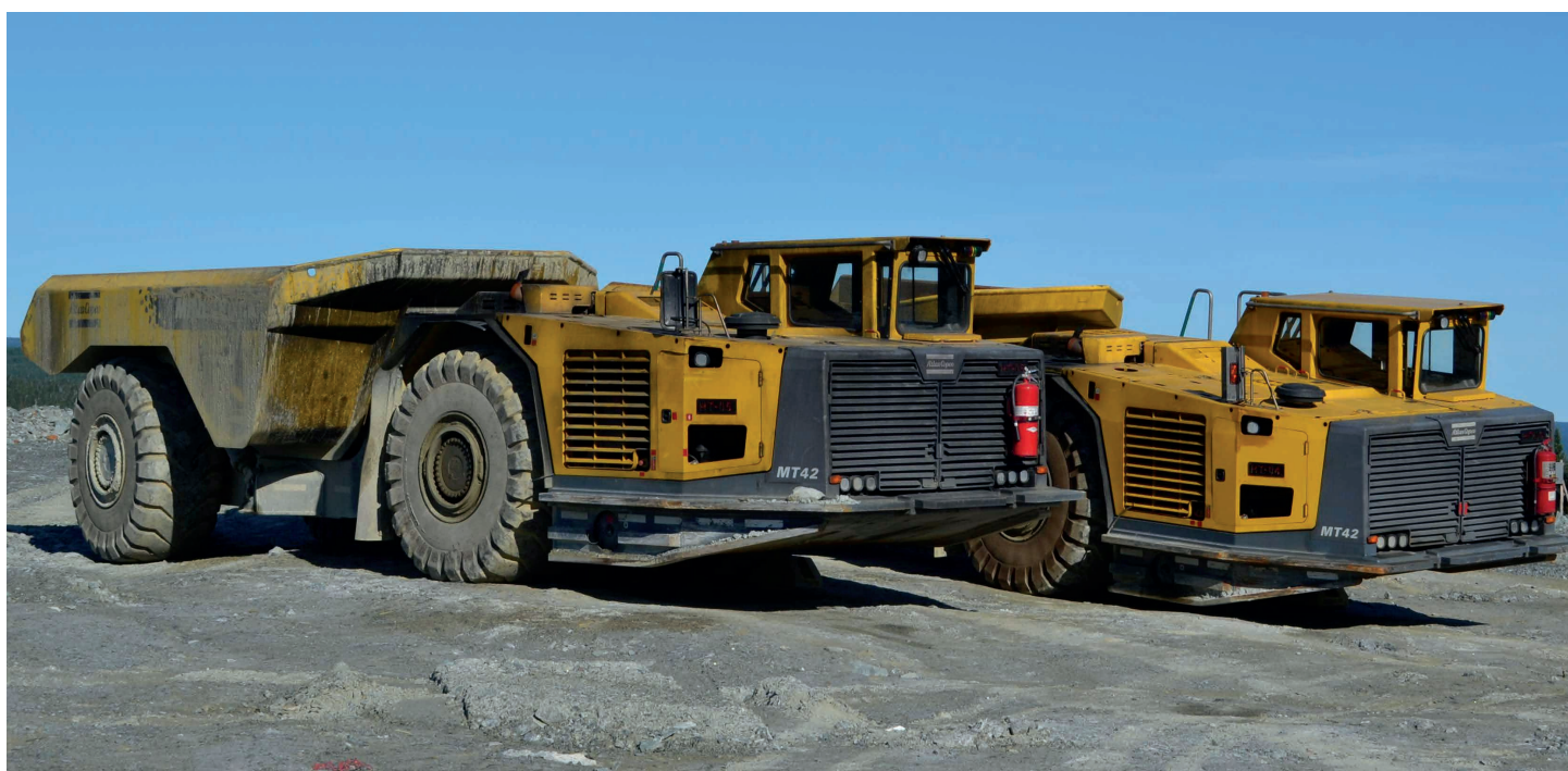
Rambler Haul Trucks, Ming Mine Site Photo Credit - Rambler Metals and Mining Canada Limited
