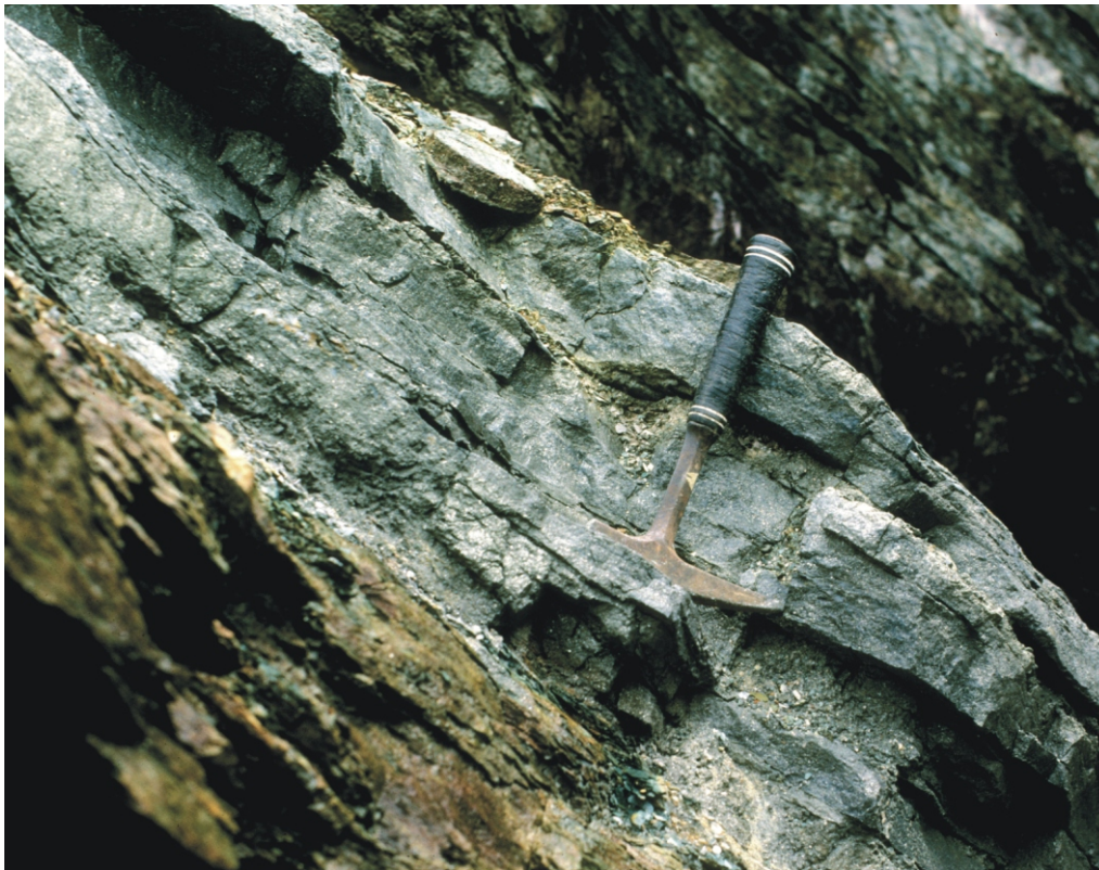
Plate 25. Pyrite and minor chalcopyrite lens within chlorite schist, Little Bay Mine glory hole.
